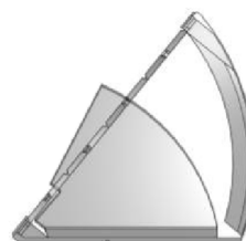
The rotating rigid cells with zero poisson ratio design
