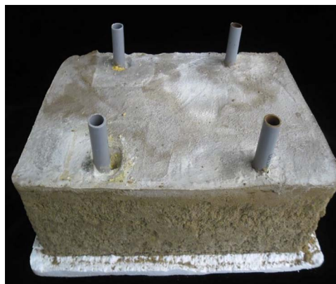
Figure 1. Sand specimen after biocement treatment with bacterial cultures and cementation solution
