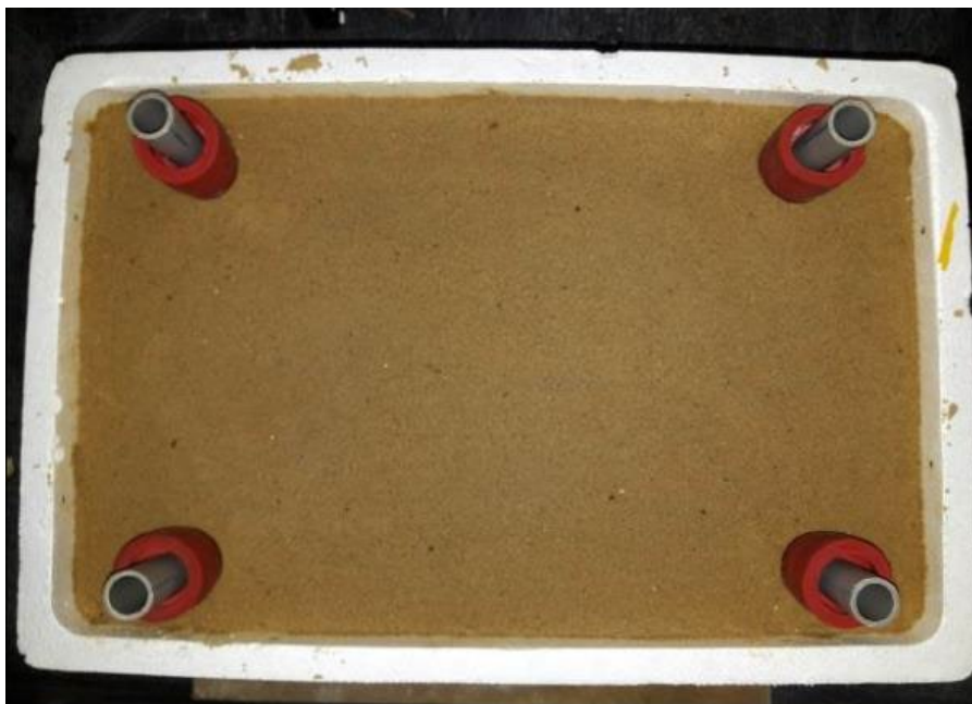
17 Figure S5: A digital image displaying the two-stage soil biocement injection treatment under 18 laboratory-condition.
