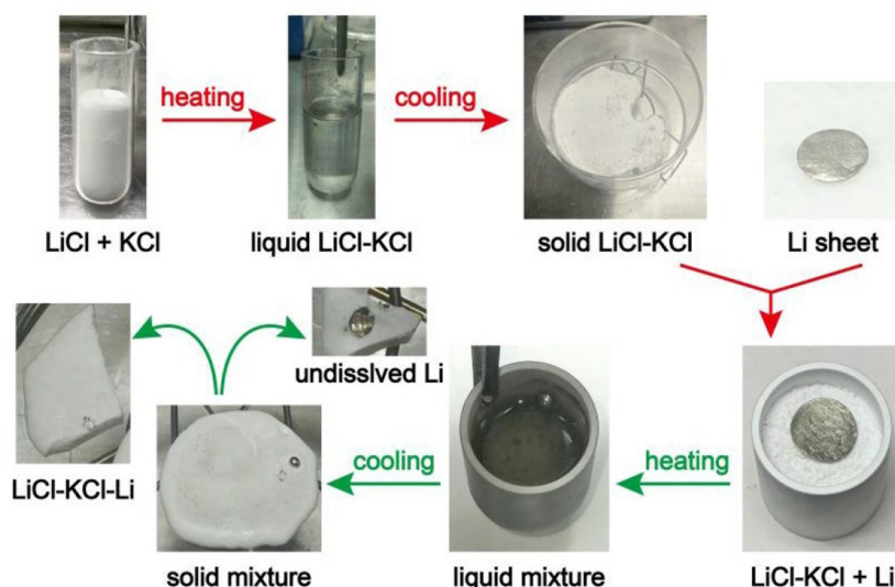
Figure 1 Preparation flow chart for LiCl-KCl and LiCl-KCl-Li samples
