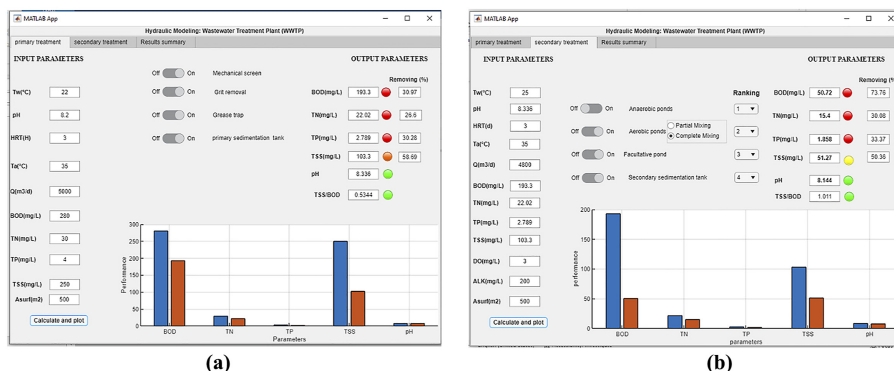
Figure 2. (a) The interface of the MATLAB App Designer model for primary treatment (b) The interface of the MATLAB App Designer model for secondary treatment
