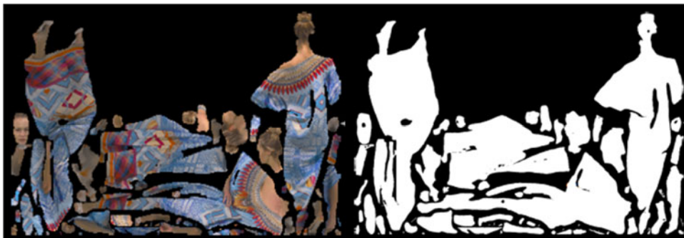
Fig. 8. Texture (left) and occupancy (right) images for the first frame of Longdress using V-PCC.
