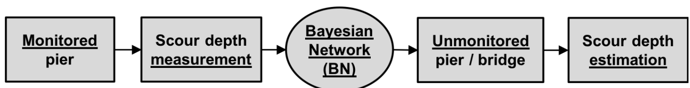
Figure 2: Schematic rationale of the scour hazard model
