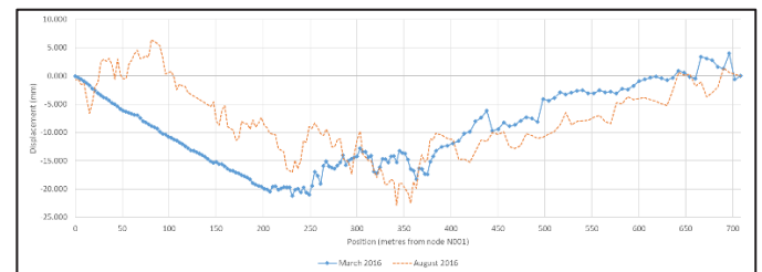
Figure 3.2 Measured displacement of the Dover sea wall in March and August 2016.
