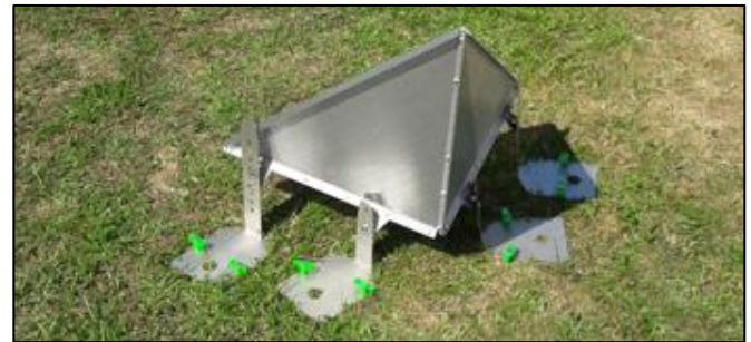
Figure 4.1 Ground mounted 50cm corner reflector
