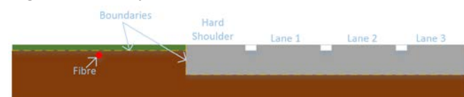
Figure 9 Directly buried fibre cable
