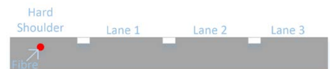
Figure 8 Slot cut deployed fibre cable
