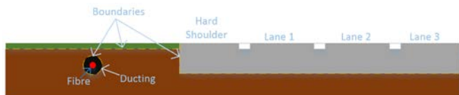
Figure 10 Directly buried ducted fibre cable
