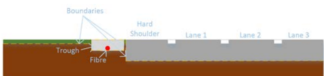
Figure 11 Fibre cable in a concrete trough
