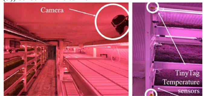
Figure 3 Picture of a camera and TinyTag (Temperature (3)) sensors in the tunnel
