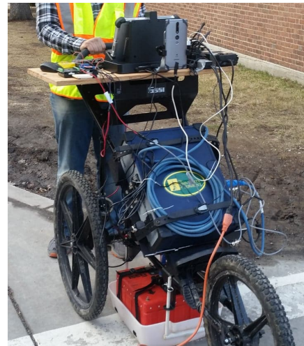
Figure 1 Ground penetrating radar integrated with augmented reality device.
