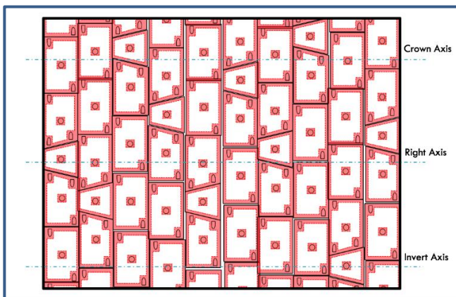
Figure 4b: A representative view on the tunnel lining demonstrating the significant quantity of surface area occupied by no-drill zones.
