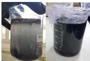
Figure 2: Aqueous dispersion of GNPs (the product is G2NanPaste supplied by Nanasa) before (left) and after 2 hours of sonication (right), in the presence of PCE.
