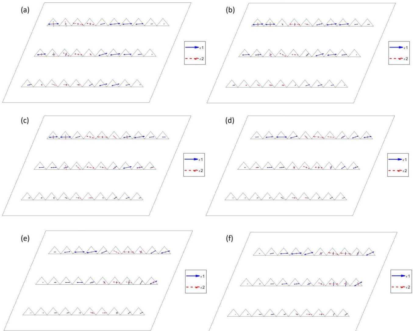
Figure 8 Principal strains mapped across the arch barrel of bridge CFM-5 for a typical 2-carriage train travelling on the northern (top) track, for cases where the axle loads are applied directly above (a) rosette 3, (b) rosette 4, (c) rosette 5, (d) rosette 6, (e) rosette 7, and (f) rosette 8; \epsilon_1 is compressive and \epsilon_2 is tensile
