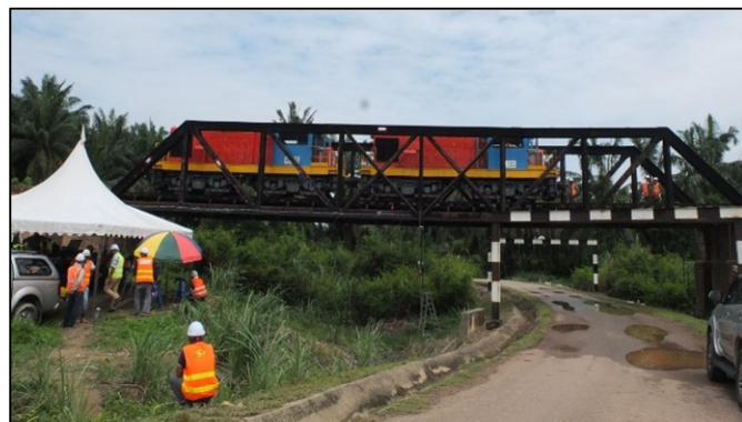
Figure 6 Example of Load Test Arrangement: Case 13 - Double Locomotive Static Test 25 m from Abutment A
