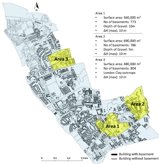
Figure 7 Case study areas for thermal interaction comparison between basements and the natural subsurface (© University of Cambridge)
