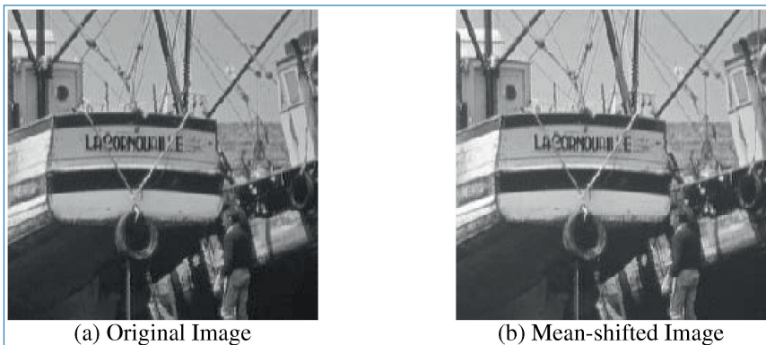
Figure 11.10. Comparison of “Boat” images: (a): original image; (b): mean-shifted image with MSE = 210 and SSIM = 99\% . [WBSS04]
