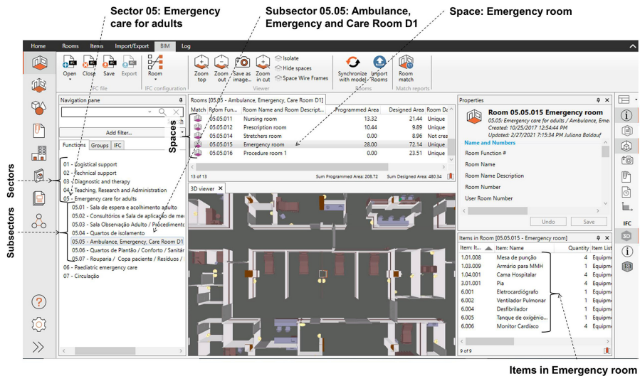
Figure 6. Modelling of functions, spaces, items and the digital model of the new ED
