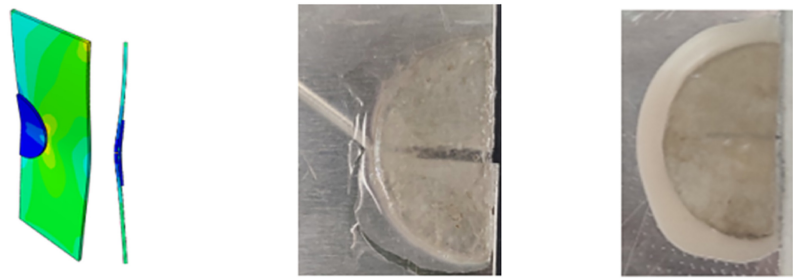
Cracked Specimen with Semicircular patch ( R_p = 17\text{mm} ) (d)
