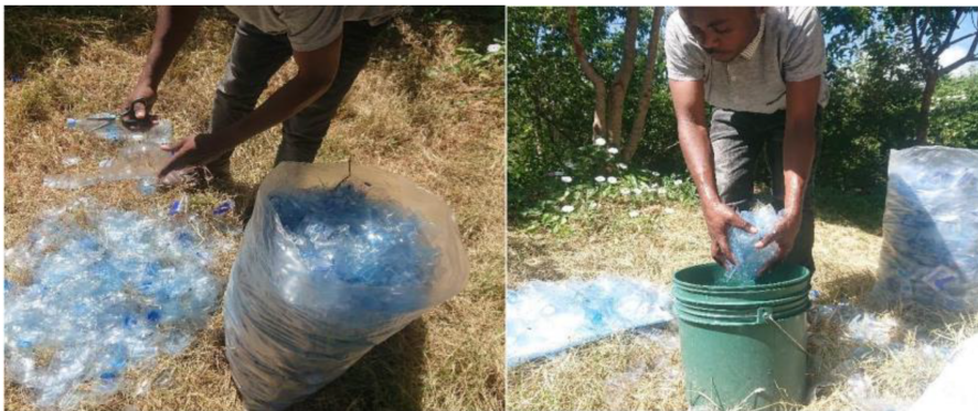
Plate 1. Waste plastic bottles collection, slice and washing process
