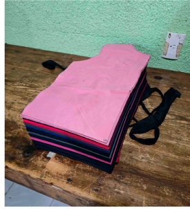
(a) Fabric pieces (eight light and five dark colors) for a large size pants after cutting and before separation process
