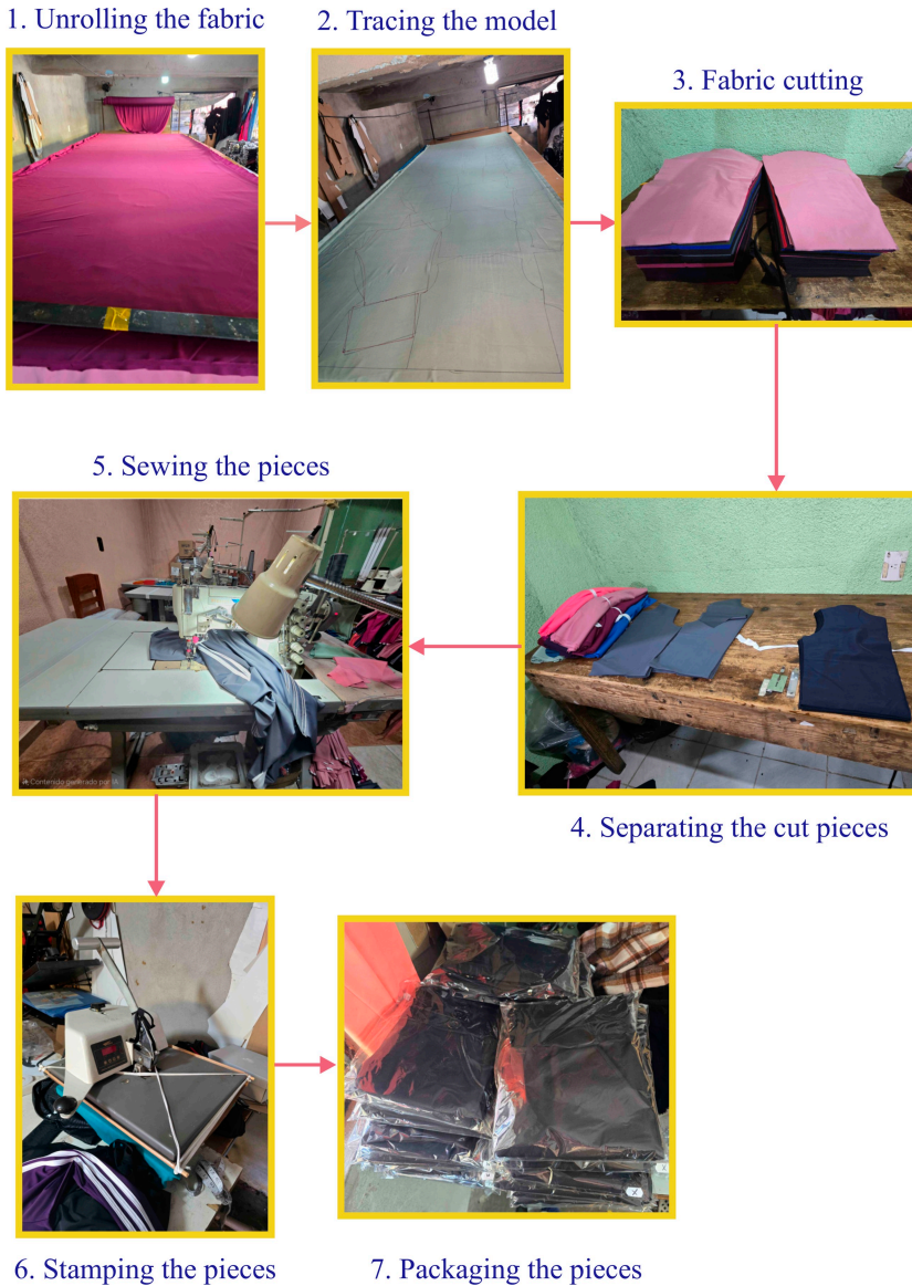
Figure 3. Manufacturing process of women sports pants in the SME Source: Authors' own work
