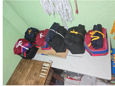
(d) Several batches using color code strips for pants sizes (yellow for medium size and white for large size)
