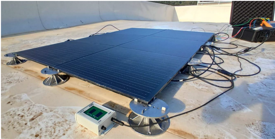
Figure 6. Experimental thermal analysis on the selected BIPV floor tiles. Source: Authors' own work
