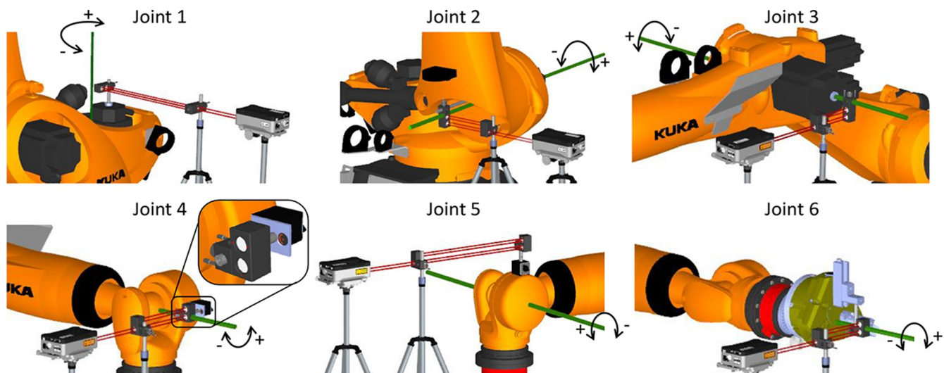
Figure 3 Mechanical fixtures used to mount the angular optical setup on robot joints
