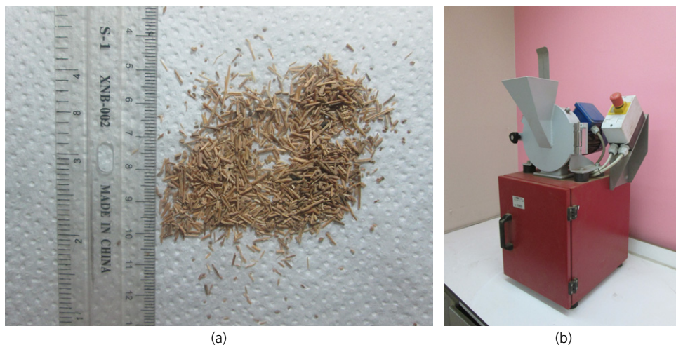
Figure 1. Appearance of hammer-milled DPFs (a) and machine used (b)
