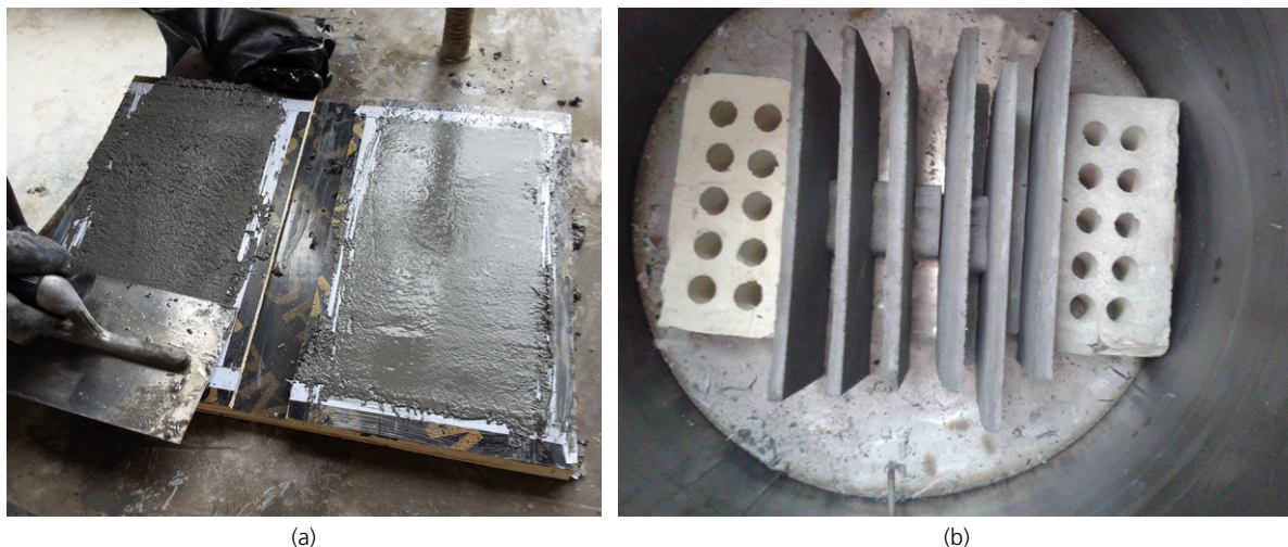
Figure 3. Typical specimen appearance after casting (a) and early age boards installed inside the carbon dioxide curing chamber ready for carbonation (b)
