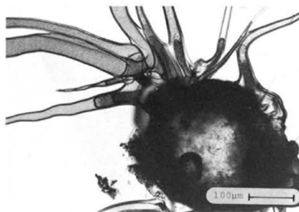
Fig. 1. Silicate garden seen under the microscope, by immersing a small crystal of dried ferrous sulphate heptahydrate in 20wt% sodium silicate solution ( \text{SiO}_2/\text{Na}_2\text{O} = 3 ); the crystal appears as the dark sphere from which the fibrils grow
