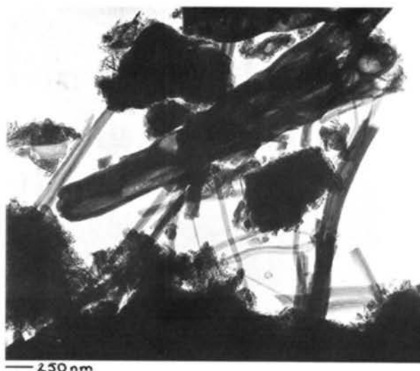
Fig. 5. TEM micrograph of the reaction product from a PFA–20wt% lime–4wt% gypsum specimen cured for 18 hours at 90°C in 100% relative humidity
