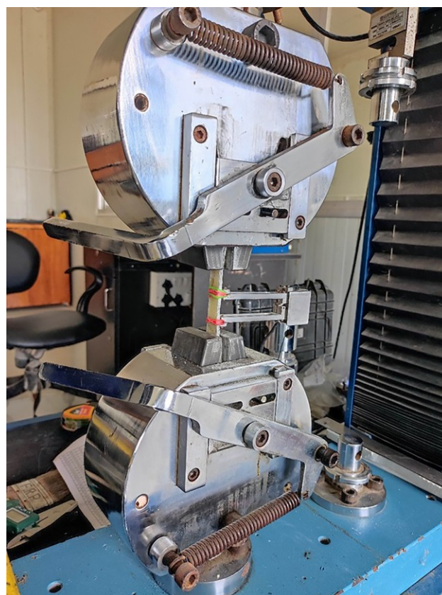
Figure 5. Specimen attachment with extensometer arrangement
