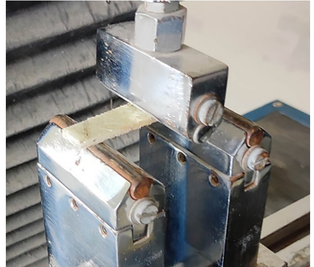
Figure 8. Specimen subjected to three point bending in UTM apparatus
