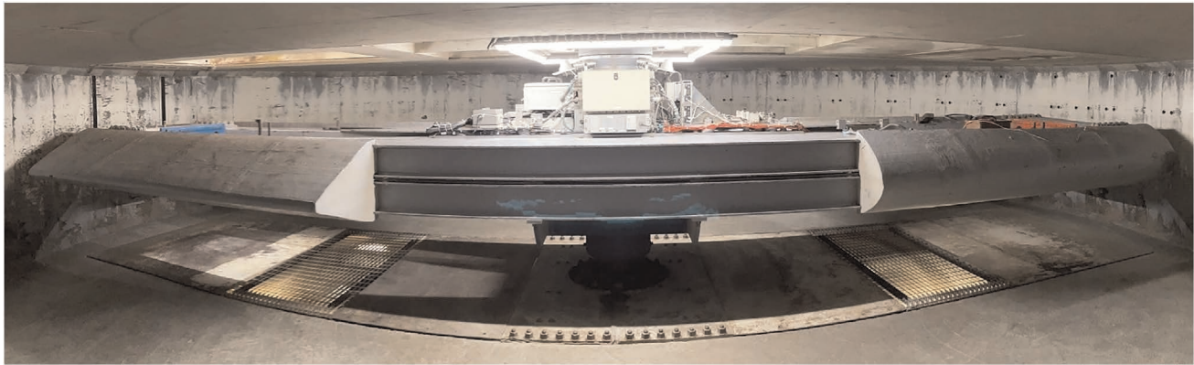
Figure 3. Turner beam centrifuge (10 m in diameter) at the Schofield Centre, University of Cambridge
