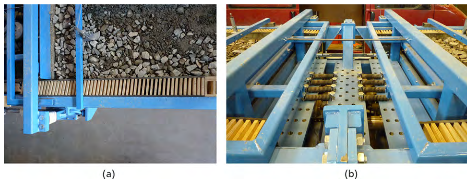
Figure 3. (a) Structure of side walls in soil containers of the IBS. (b) Springs between the frame of the test device and the loading plates
