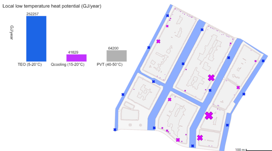
Figure 4. Identification of local low temperature heat potential in GJ per year in Leliegracht neighbourhood (Dang, 2024)
