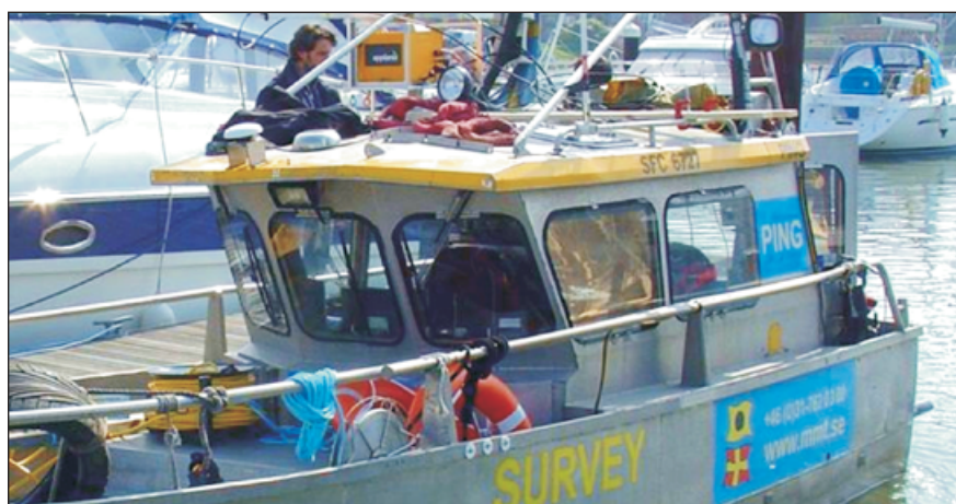
Smaller bridges over fast-flowing rivers cannot be examined with boat-mounted sonar equipment
