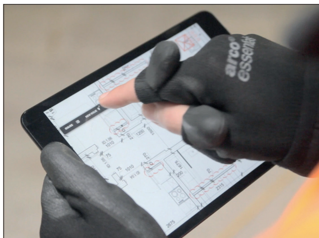
Figure 14. The red line application, which enables an operator to conduct red-lining using a tablet interfacing directly with the central building information modelling database
