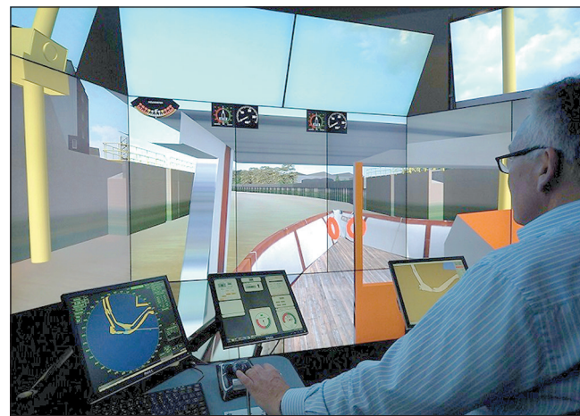
Figure 10. The project building information model was also used for river navigation simulations at HR Wallingford (Environment Agency)
