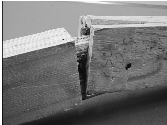
Fig. 3. Failure of an in-line beam-to-beam connection tested in four-point bending
