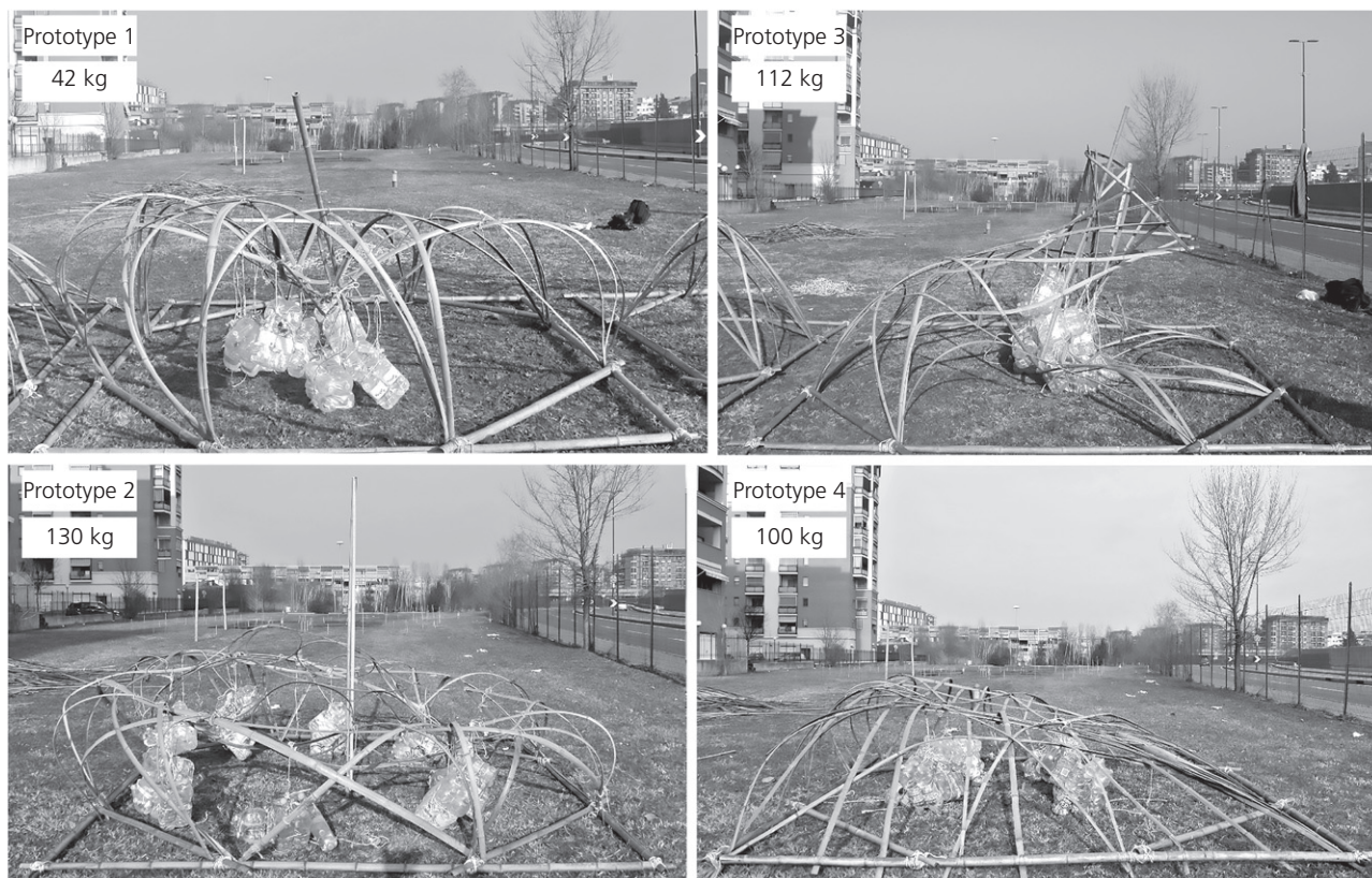
Figure 3. Prototypes at failure
