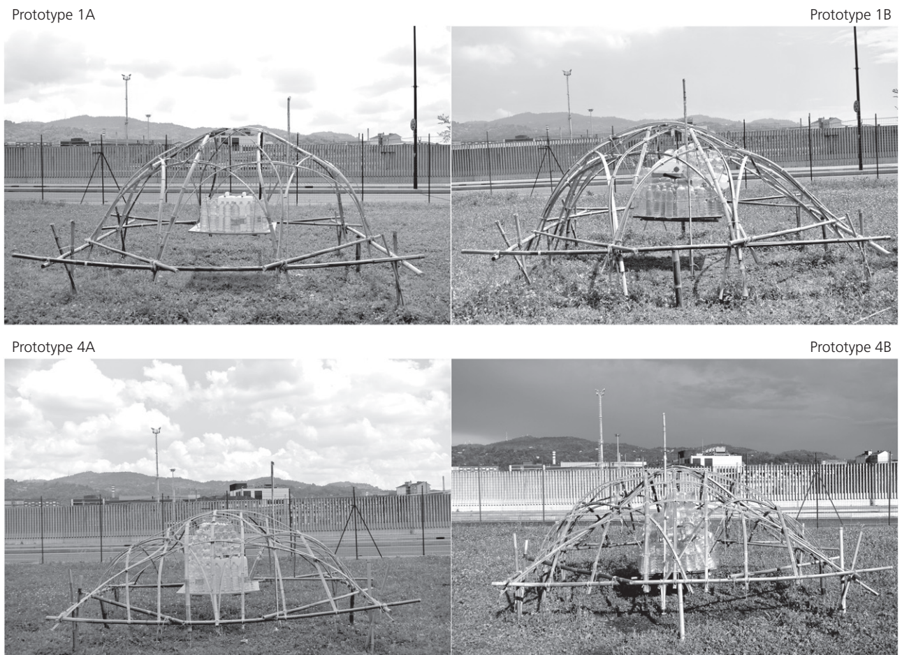
Figure 7. Comparison of loading and deformations in prototypes 1A and 4A with their respective 'enhanced' versions, 1B and 4B
