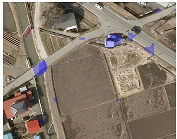
Figure 8. Examples of false detections involving undamaged bridges. These include cases where undamaged bridges were misclassified as damaged, or road segments were incorrectly detected as undamaged bridges
