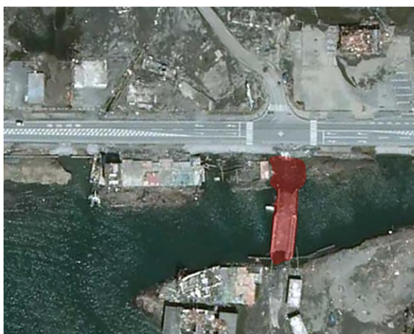
Figure 7. Segmentation results for damaged bridges with detection failures caused by flooding or structural collapse. When parts of a bridge become unobservable due to inundation or the loss of structural components, those regions may not be detected
