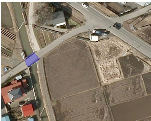
Figure 8. Examples of false detections involving undamaged bridges. These include cases where undamaged bridges were misclassified as damaged, or road segments were incorrectly detected as undamaged bridges
