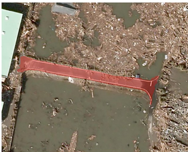
Figure 6. Segmentation results for damaged bridges were partially detected due to debris accumulation. In cases where large amounts of debris extend beyond the bridge deck or float on the surrounding water surface, parts of the bridge may not be detected
