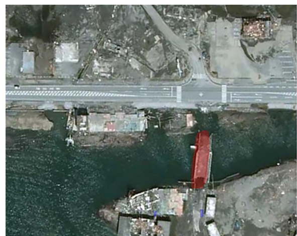
Figure 7. Segmentation results for damaged bridges with detection failures caused by flooding or structural collapse. When parts of a bridge become unobservable due to inundation or the loss of structural components, those regions may not be detected
