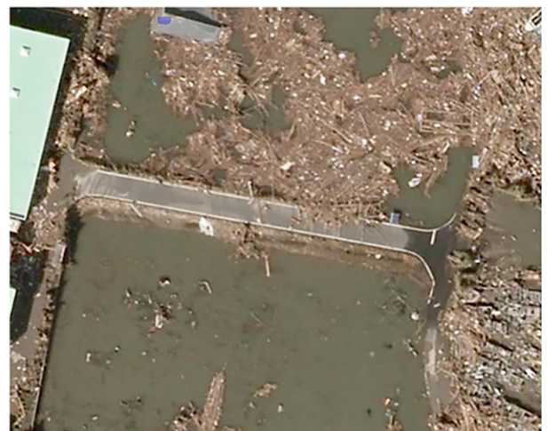
Figure 6. Segmentation results for damaged bridges were partially detected due to debris accumulation. In cases where large amounts of debris extend beyond the bridge deck or float on the surrounding water surface, parts of the bridge may not be detected
