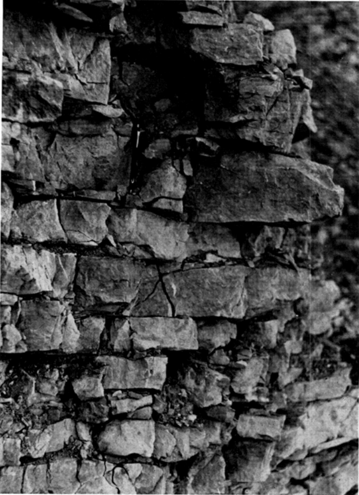
Fig. 1. Red and variegated nodular limestone with clayey beds (Upper Cretaceous), zone of rock above the slip surface
