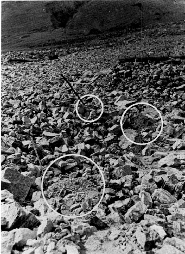
Fig. 2. Lumps of bentonitic clay (in white circles) on slide debris from slip surface
