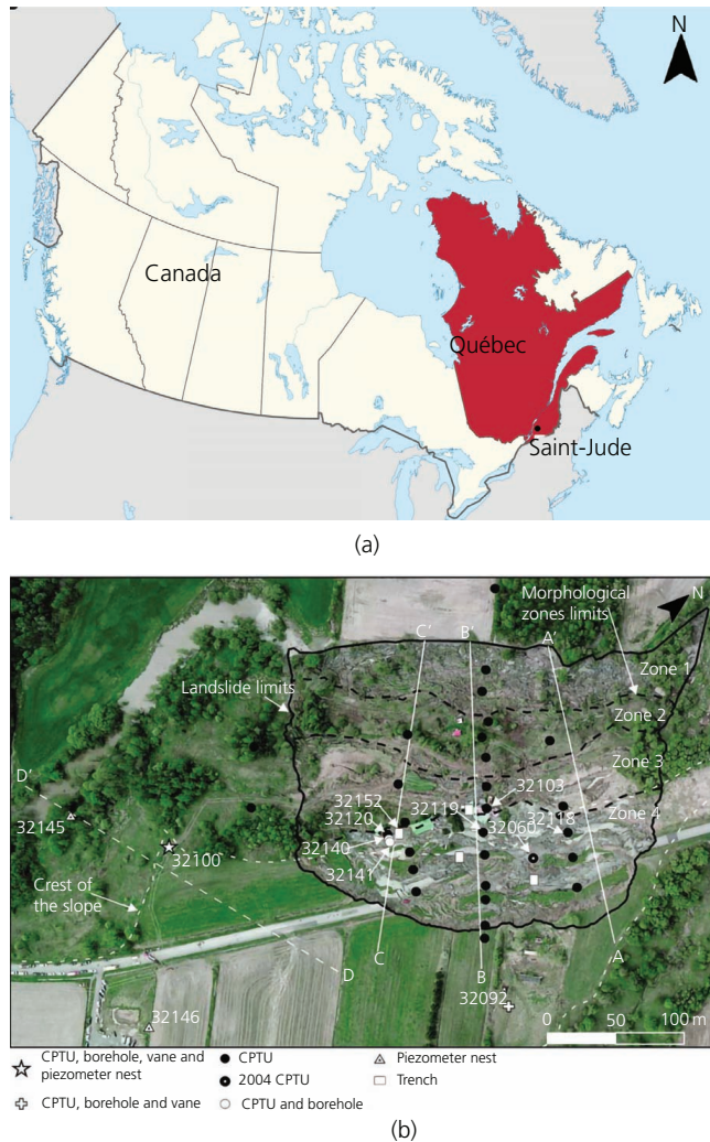
Figure 2. Saint-Jude landslide: (a) location of Saint-Jude; (b) aerial view of the landslide (modified from Locat et al. (2017)). CPTU, cone penetration test with pore water pressure measurement
