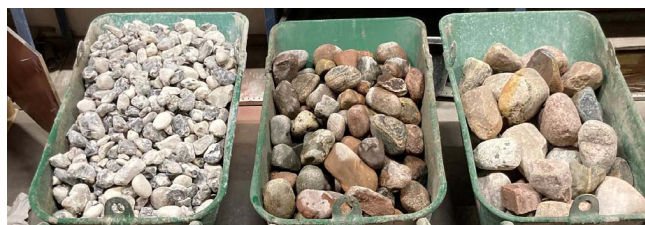
Figure 3. The three coarse-grained materials tested. From left to right: d_{15} = 35, 75 and 110 mm
