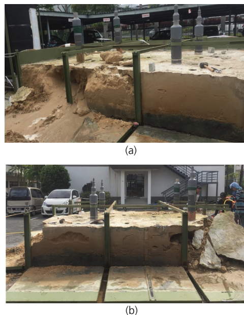
Figure 1. A sandbox ( 10 \text{ m}^3 ) was subjected to bio-cementation treatment. (a) Front view of the treated soil mass after an outdoor trial treatment; (b) rear view of the treated soil mass
