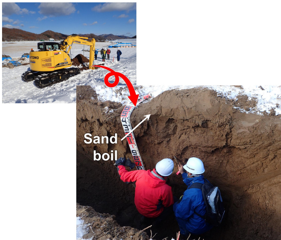
Figure 10. Progress in observation of soil profile on test trenching
