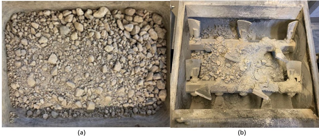
Figure 1. (a) Unbound RCA and RG mixture. (b) Blending apparatus
