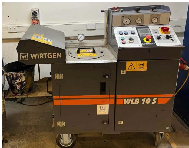
Figure 2. Laboratory-scale apparatus used to create FB
