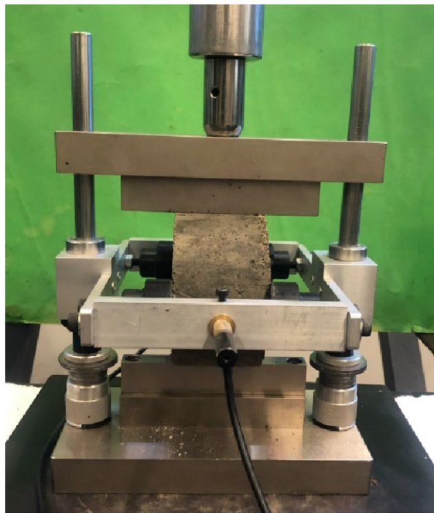
Figure 3. ITM r testing setup and sample
