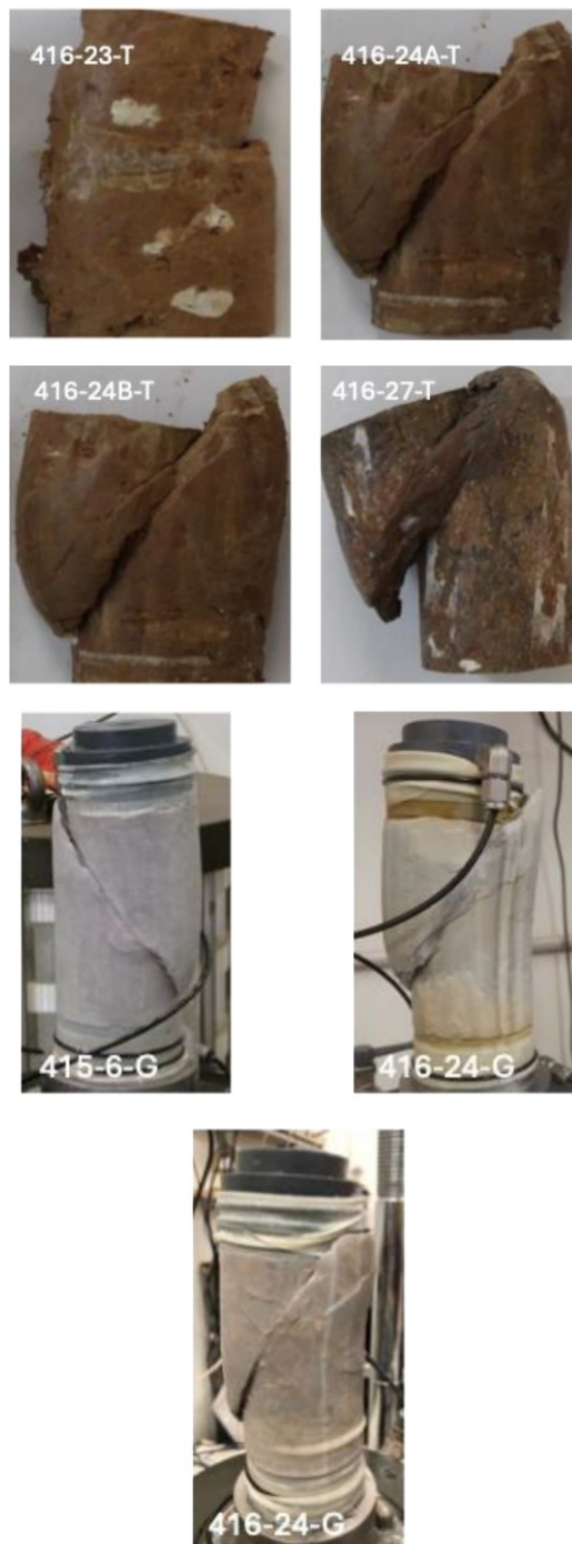
Figure 26. Photographs of sheared triaxial samples
