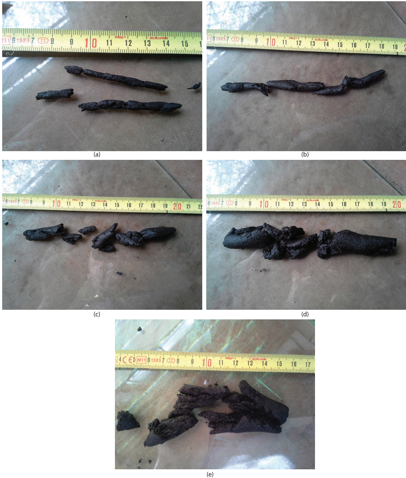
Figure 6. Failure condition of the soil threads. (a) Specimen A at PL ( d = 3 mm; F = 0.5 ; w = 578\% ); (b) specimen B at 'PL' ( d = 6 mm; F = 0.5 ; w = 85\% ); (c) specimen C at 'PL' ( d = 10 mm; F = 0.5 ; w = 597\% ); (d) specimen D ( d = 16 mm; F = 0.2 ; w = 628\% );
