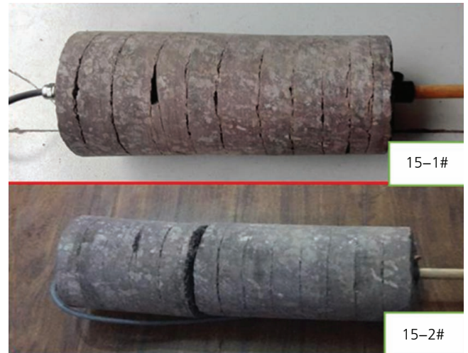
Figure 10. Examples of discing after overcoring at chainage 07+280 in TBM 697
