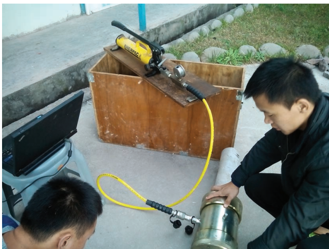
Figure 8. Biaxial test after overcoring test on the specimen
