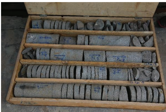
Figure 9. Core discing in the borehole drill at chainage 09 + 860.8 in TBM 696
