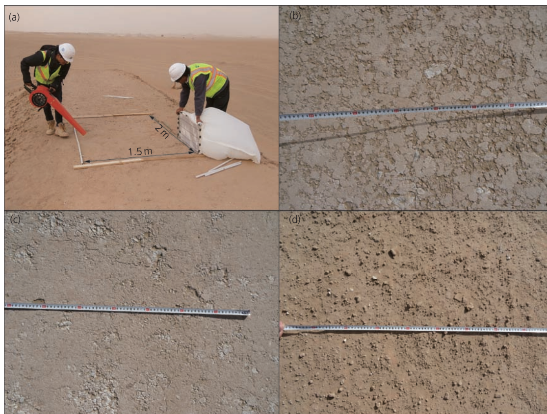
Figure 12. Sand fixation layers after wind erosion tests. (a) In situ wind erosion test; (b) sandstone–gypsum; (c) sandstone–gatch; (d) sandstone
