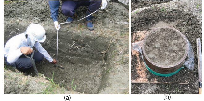
Figure 11. Block sample of the extra fill in 2011: (a) 0.5 m below of the top; (b) MDC lumps in the block
