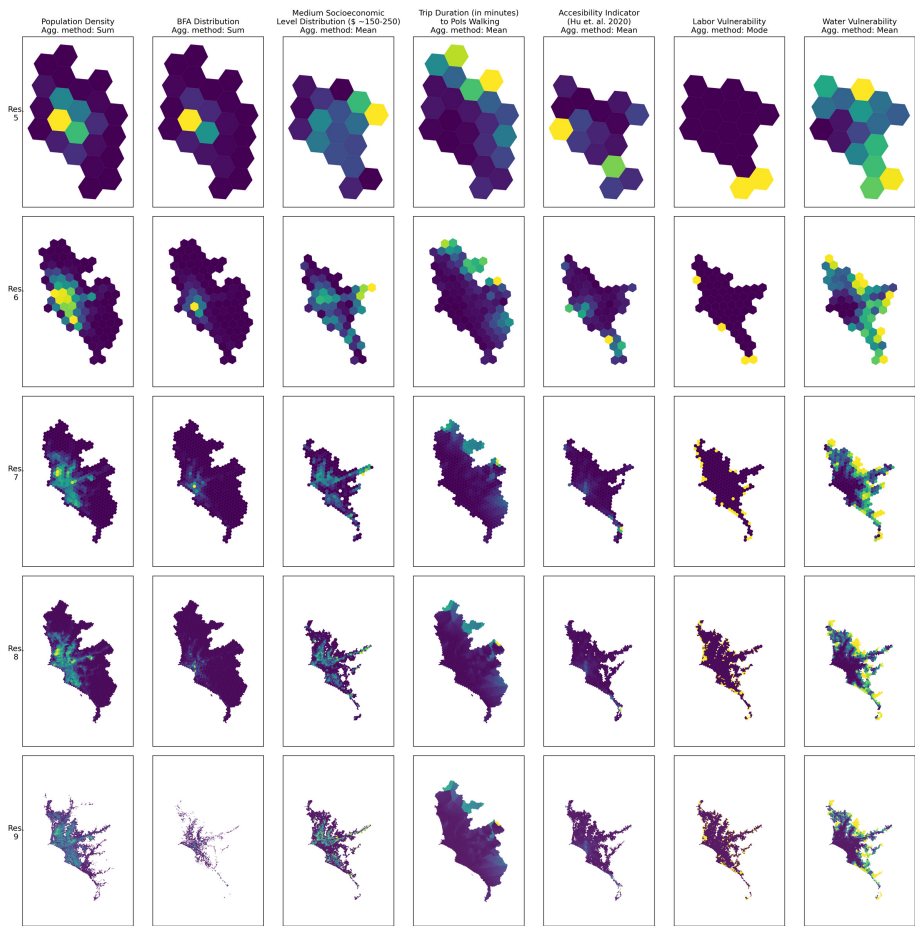
Figure A1. Resolution downsampling process. This allows to aggregate hexagons in coarse resolutions
