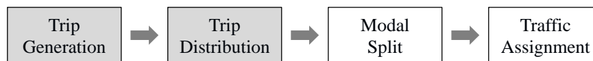
Figure 1. Trip generation and trip distribution in the four-step transportation demand forecasting model
