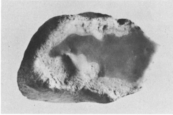
Figure III: Typical piece of Thames Valley river gravel aggregate (taken at random) and impression left by it in cement paste.
