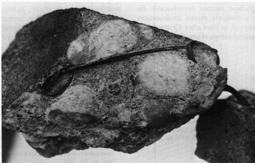
Figure III: Akwara after 42 months of embedment in concrete.
