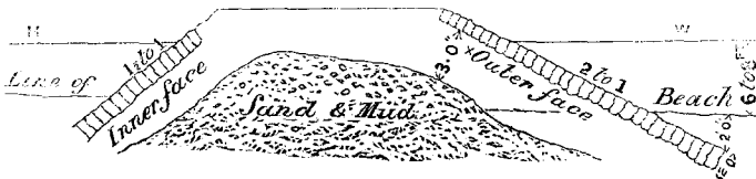
Section of Embankment in the Clontarf Estuary.
